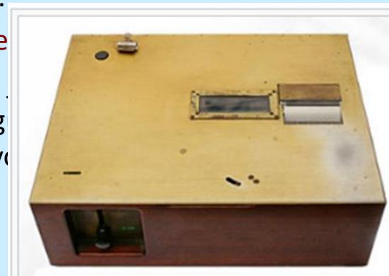
The teaching machine, a mechanical invention to automate the task of programmed learning
